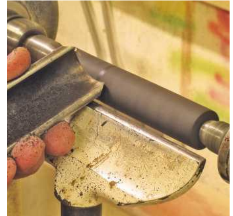
▲ Pic.21 Mount the ebony for the stem between centres and make it round with the roughing gouge. Turn the whole piece down to 18mm, the maximum diameter of the stem
